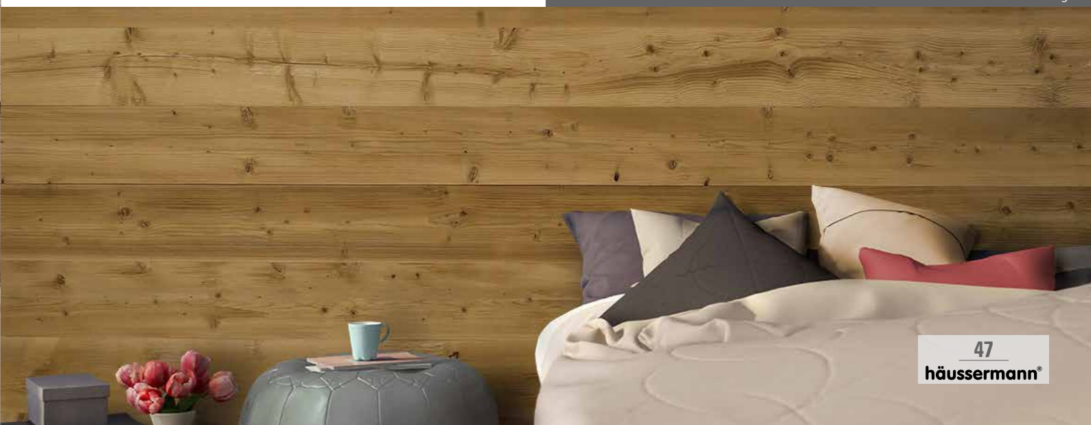
Figures: Thermally modified spruce, chopped, Neorustic Dimensions: 19 x 136 mm, 19 x 161 mm, 19 x 186 mm System length, tongue + groove all round
