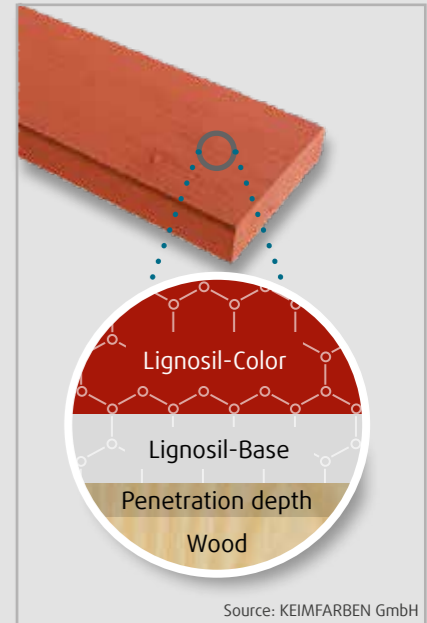
Ultra-fine silicate fillers from Lignosil-Base form a permanent bond with Lignosil-Color
