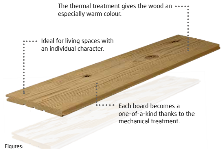
Figures: Thermally modified spruce, chopped, Neorustic Dimensions: 19 x 136 mm, 19 x 161 mm, 19 x 186 mm System length, tongue + groove all round
